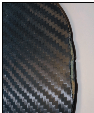
Photo 2 : Edge of seat plate splintered
